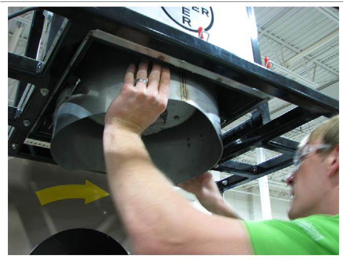
**INSERT LINER ASSEMBLY Step 1:** Lift the Liner Assembly up into the Atomizer Housing, inserting the cut-out grooves over the conduit tube and the chemical inlet tube.
