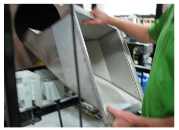
**SEED INLET TRANSITION Step 1:** Unlatch the Transition latches and remove it from beneath the Atomizer Housing.
