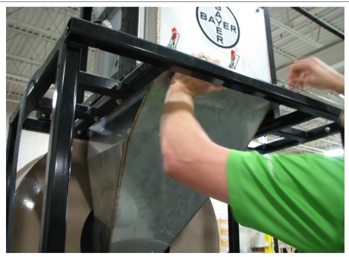
**SEED INLET TRANSITION Step 1:** Replace the Transition up underneath the Atomizer Housing and lock it in place.
