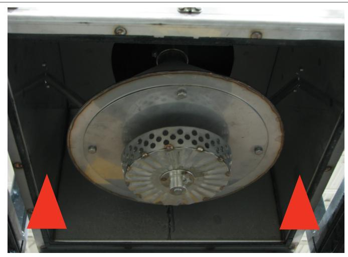
ATOMIZER HOUSING Step 1: Use a putty knife to scrape and clean the interior of the Atomizer Housing.
