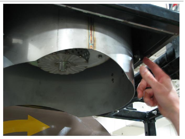
**LINER ASSEMBLY Step 1:** Push the right rubber foot in and push up on the Liner.
