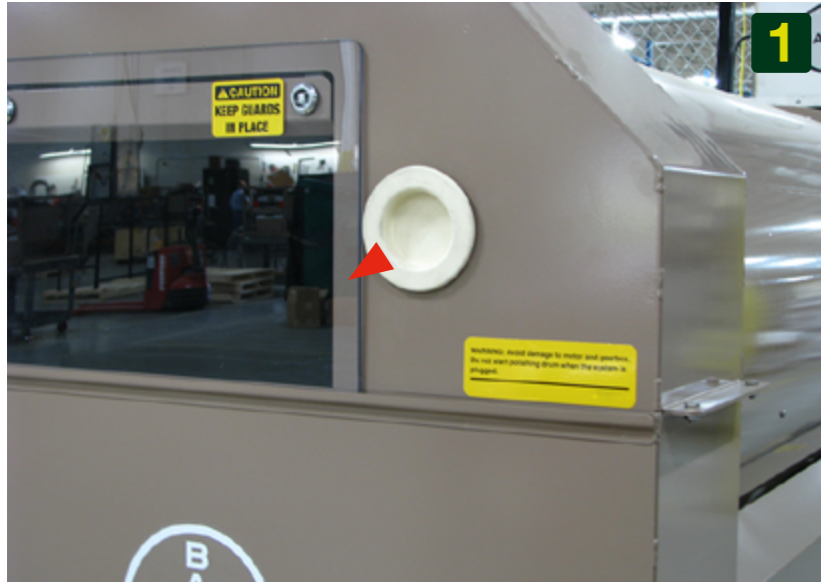
Remove Rubber Plug from Doghouse, ref.
