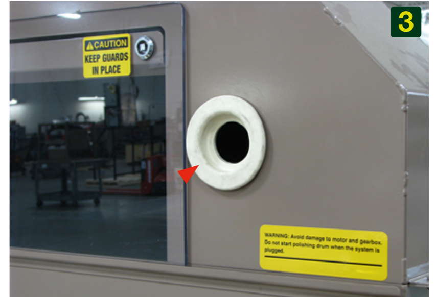
Insert the Auger Tube Seal into the Doghouse, ref.
