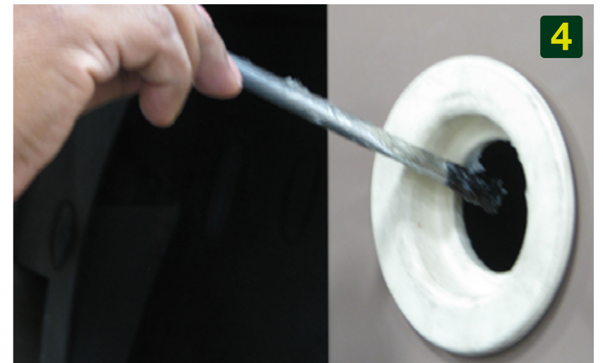
Apply Petroleum Jelly on Auger Tube Seal orifice, ref.
