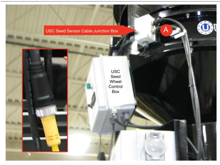
**JUNCTION BOX CONNECTIONS - USC SENSORS** The USC Seed Sensor Cable is connected to the USC Seed Wheel Control box, as shown above.
