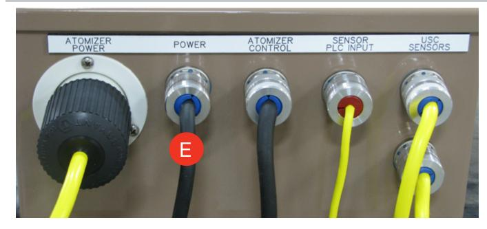
JUNCTION BOX CONNECTIONS - POWER CORD Step 1: Connect the Junction Box Power Cord E to an external 115V power source (power light illuminates green).
