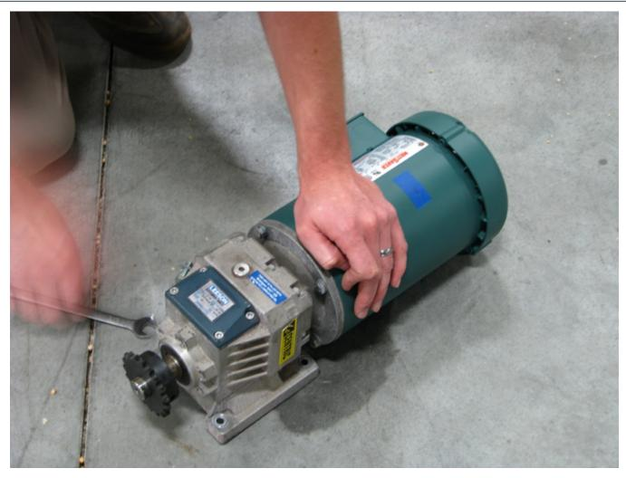
**MOTOR MOUNT Step 1:** Connect the Gear Reducer to the replacement Motor.
