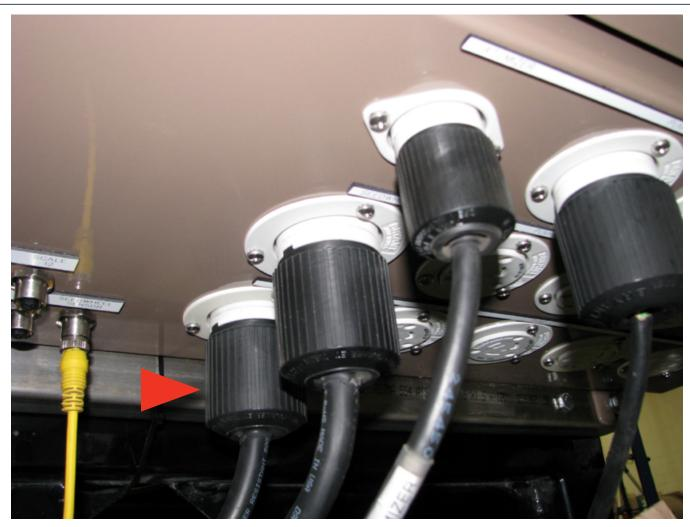
MOTOR Step 1: Plug the replacement Motor Power Cord CBL:30FT L15-20 TWIST LOCK X 4 WIRE (attached to replacement motor) to the bottom of the On Demand Main Control Panel (receptacle marked Drum Motor).
