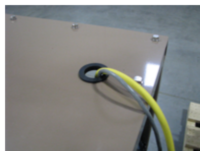
Bowl Supply Hopper Gray Load Cell Wire and Solenoid Box Yellow 10-pin Cable shipped out of Weigh Scale conduit hole top side
