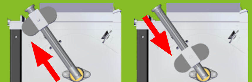
Move Counterweight Up to Decrease Trips
